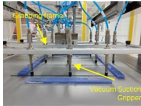
Figure 3. The photo of Vacuum and nozzle clamp on the Grabbing frame.
