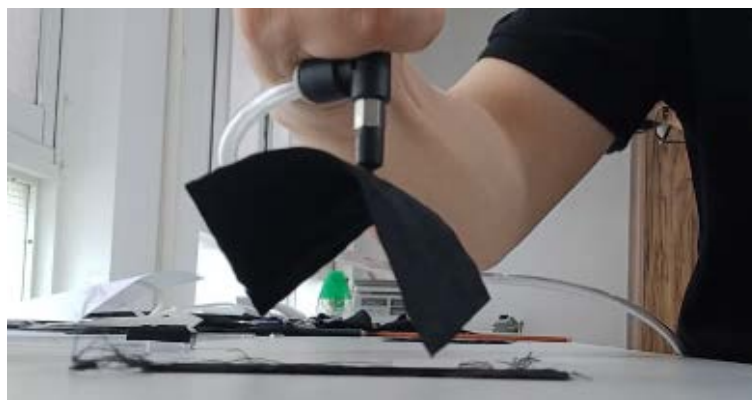
Figure 8. Photo of single grabbing test to determine the grabbing pressure and radius of vacuum grabbing pressure theoretical circle.
